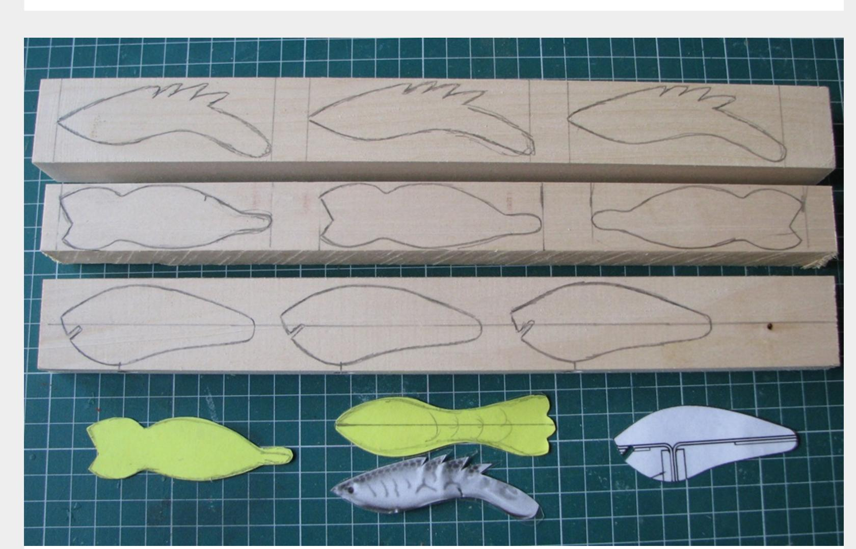
The top basswood blank (1" thick x 1-1/4" wide) shows crayfish lure designs that will be cut out on the bandsaw. The middle basswood blank shows hula popper lure designs, which will be hand carved. The bottom basswood blank shows crankbait lure designs. Rip the blank to 5/8" thick x 1" wide, drill a 5/16" hole in the bottom and saw cut a 1/16" kerf about halfway through from the bottom for rigging a weight and hook attachment loops.
