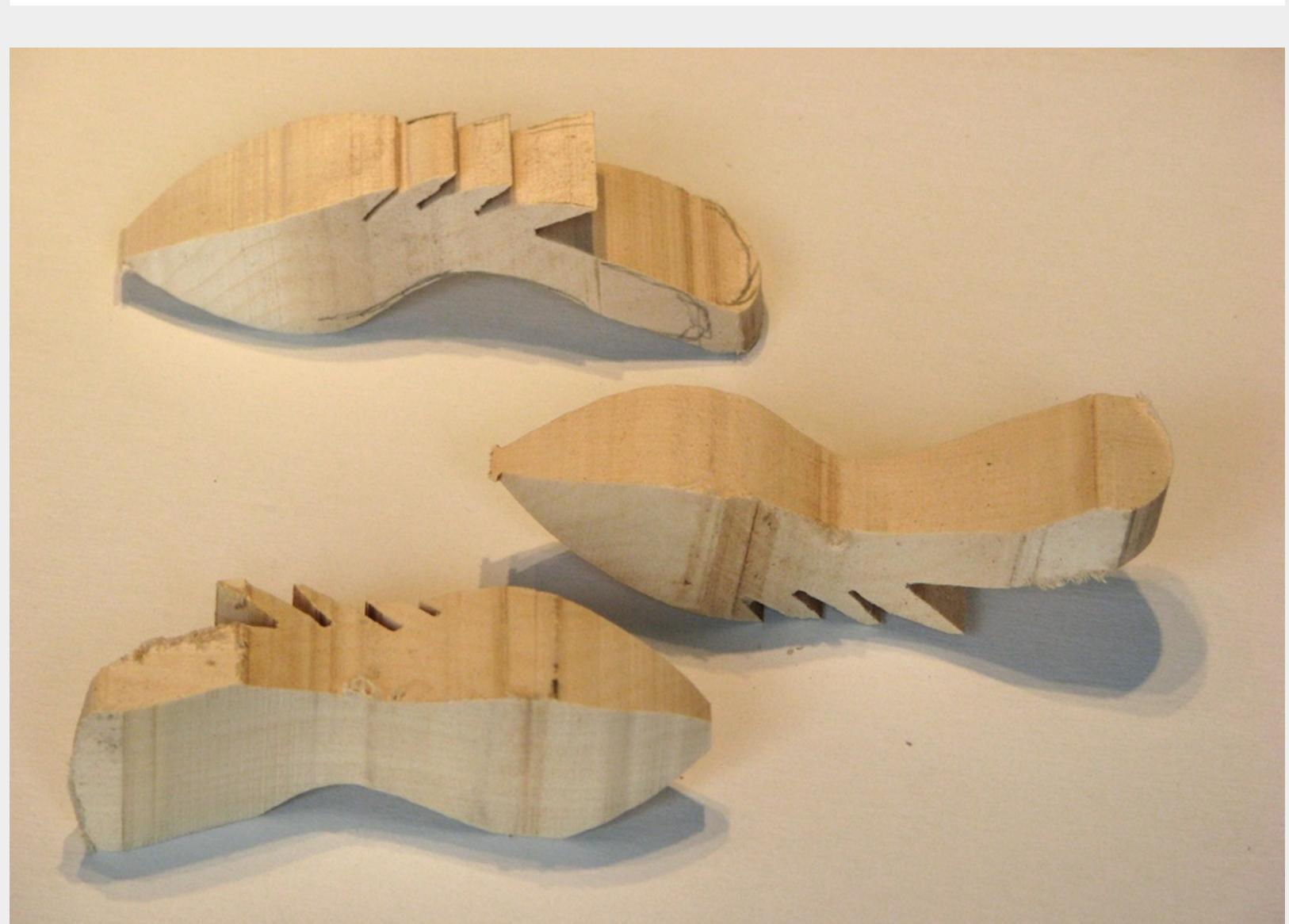
The crayfish blanks were cut on the bandsaw. Later, a hole is drilled in the bottom to add weight.
