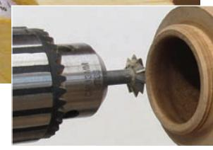
60° rotary cutter in Jacobs chuck
