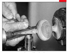
**5. Turn the finial** after regluing the half-balls back together.
