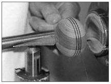
**6. Disguise the join** with lines burned by a stainless steel wire.
