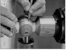
**2. Reference line** across the high point will help reassemble the ball later.
