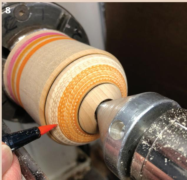
Add chatter marks between the burn lines. The author uses colored pens to highlight the chatter work. Apply the tip of the pen to the wood and slowly rotate the blank by hand or on the lathe's lowest speed setting. Note the color bands on the blank where the author experimented with colors.
