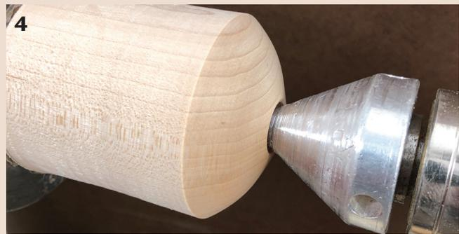
With the tailstock for support, shape the underside.
