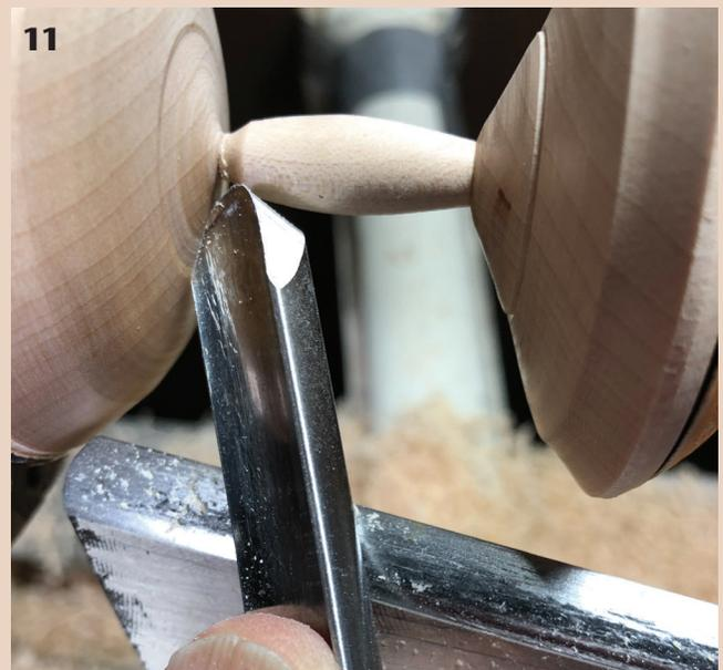
Use a detail gouge to remove the bulk of the waste material around the stem. The author switches to a parting tool for final shaping, presenting the tool edge for a slicing cut, rather than scraping cut. Return to the detail gouge to part the top.
