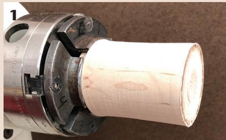
Bring a blank to round, cut a tenon on one end and mount the blank in a scroll chuck.
