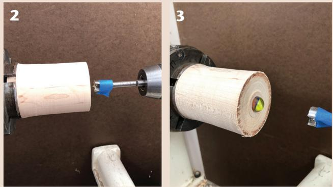
Use a Forstner-style bit in a drill chuck to cut a recess for your marble. The recess should be half the marble's diameter and the fit should be snug.
