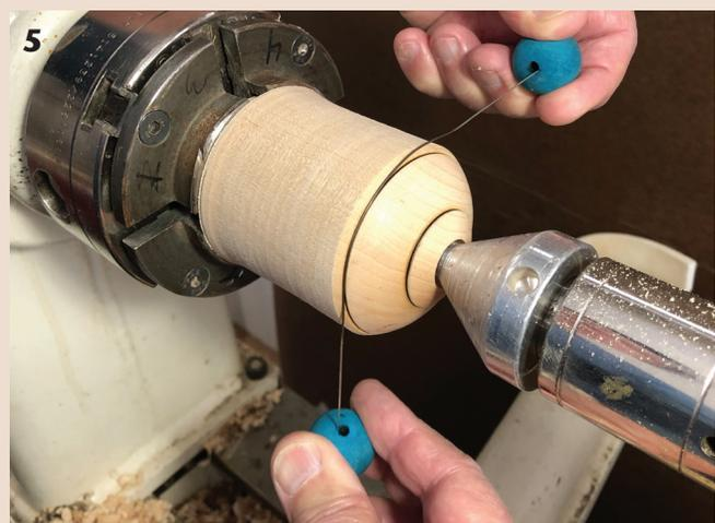
Add burn lines with a wire. A shopmade burning tool is easily made with a short section of wire (a guitar string works well) with beads for handles. Never wrap the wire around your fingers or hands.
