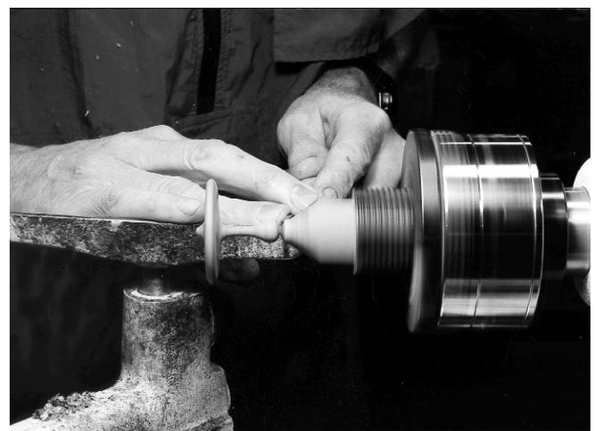
The final shape of the point on which the top spins is done after the tail stock is removed, above left. Then a skew is used to refine the top and part the piece from the lathe.
