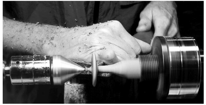
After turning the rectangular blank to a cone shape, above left, the author epoxies it into a hole bored in the disk and begins to refine the shape of the top. The stem protrudes only a half-inch below the disk. Photos by the author.
