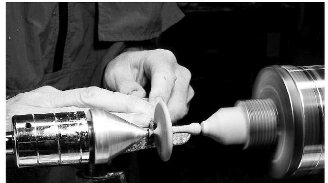
Rosand shapes a small bulbous end on the top of the stem, above left, then refines the shape of the point.
