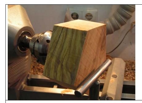
Here the blank is mounted on my lathe. I pivot the head out 22.5 degrees so that I can have full unrestricted access to the base of the bowl. I typically turn these type of bowls at 750rpm but you should use whatever lathe speed you are most comfortable with.
