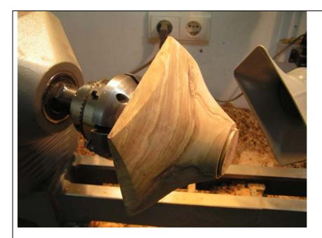
Here the outside of the bowl is completed. The spigot for the chuck has been turned and the outside of the bowl is ready for sanding. I usually power sand the outsides of these bowls but care is needed. Ensure that the sanding pad is tilted at least 25 degrees from the vertical to ensure that you don't snag the points. If you are not happy about power sanding you can sand by hand but watch the points. I lock the spindle at this stage and mark the 6 o'clock position on the chuck spigot.
