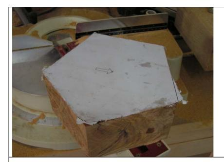
Here the blank is trimmed to shape and ready for mounting on the lathe. As you can see the paper can tear as the chop saw cuts. This is not a problem as it is the laser line that matters. This cutting stage is important and accuracy is the key. If all the sides are not the same length you can end up with a lop sided pentagon and uneven rim thickness.
