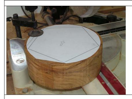
Here the blank is on my chop saw. Using the laser I line the blade up with the line of the pentagon on one side of the template. Now all you need to do is cut the first side. Rotate the blank check that the laser is still on the line and the saw hasn't moved, mine occasionally does as depending on the number of sides as you may not be exactly on a locking indent.
