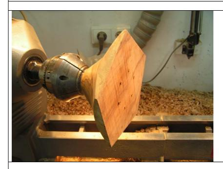
Here I have turned the bowl over and mounted the spigot in the chuck so that the mark is now in the 12 o'clock position. The reason for this is to make up for any slight offset of the chuck. Having removed the faceplate ring and the bowl is ready for hollowing the inside.
