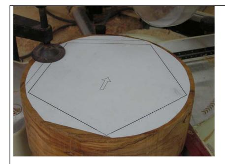
Here is the blank to start with. This is a piece of Olive that measures 9" (200mm) in diameter and 31/4" (80mm) thick. The blank does not need to be round it can be any shape. Here I have created a pentagon using MS Visio on my PC. Note the arrow added to the print out to show the centre of the pentagon. The template is temporarily glued to the blank using spray mount adhesive and the centre of the shape is marked using an awl.
