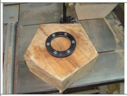
I use a faceplate ring that fits on the jaws on one of my chucks. This particular one has an inside diameter of 50mm. I use this type of ring so that I don't have to change the chuck as it is important that everything registers or you can end up with a lopsided bowl.
