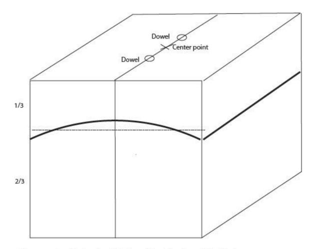
Draw arc to split the line 1/3 down from the top of the block Radius of Arc is equal to the diameter of the vessel.
