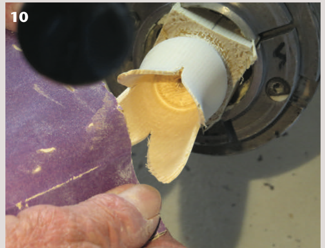
Use rolled pieces of abrasive to sand the interior. With the lathe off, sand the edge of each petal.
