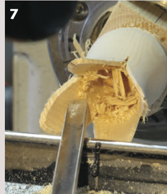
7 Use a spindle gouge to turn the interior, working down in 1/2" sections.
