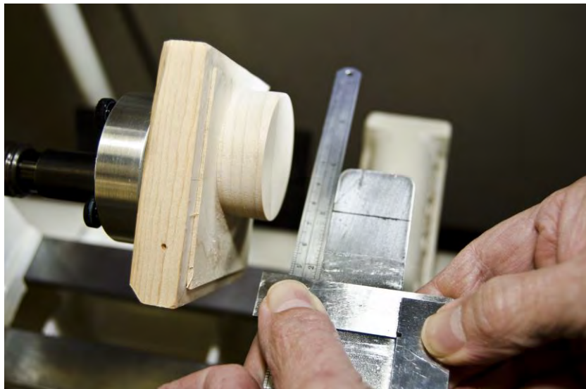
Figure 10 – Using a ruler to position a small square at the proper radius cut distance from the turning axis that's marked on the tool rest
